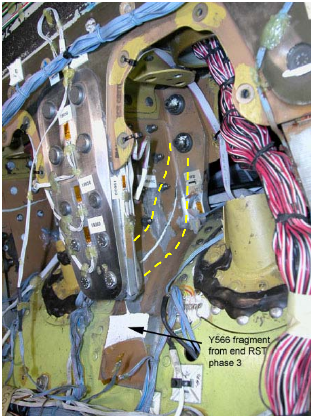
Figure 11: Overview of the failure of the Y566 stub at 79% RST load following simulated failure of the Y598 and Y590 stubs.
