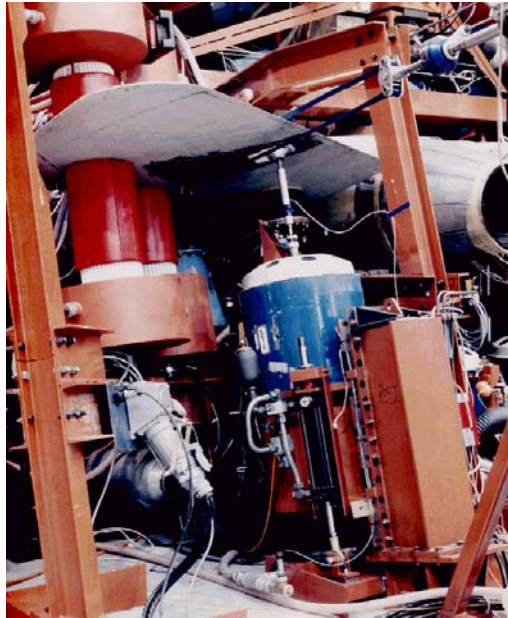
Figure 3: Rolling sleeve airbags (red) and electromagnetic shaker (blue) in place on the horizontal tail
